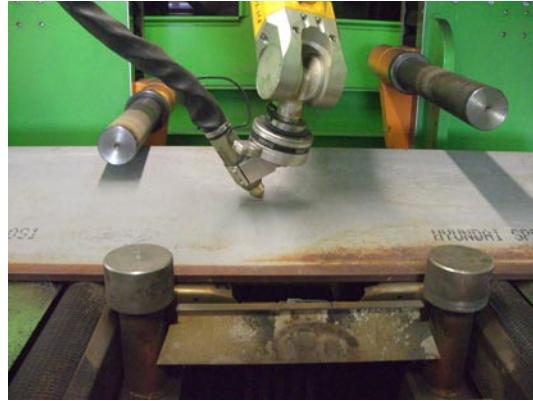
Positive, cutting angle=+40°
