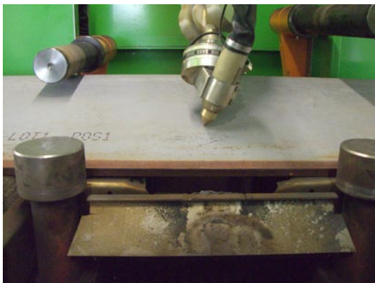
Neutral pose, cutting angle= -30^\circ
