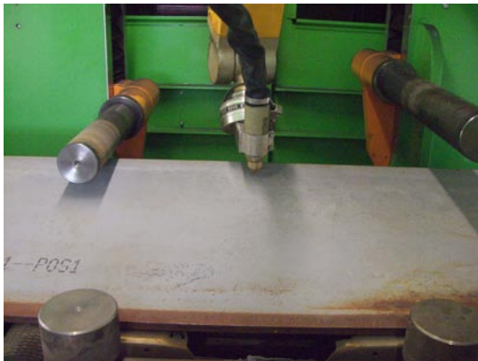
Neutral pose, cutting angle= 0^\circ
