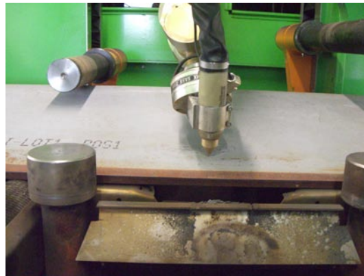
Neutral pose, cutting angle= 0^\circ
