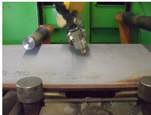
Neutral pose, cutting angle= +30^\circ
